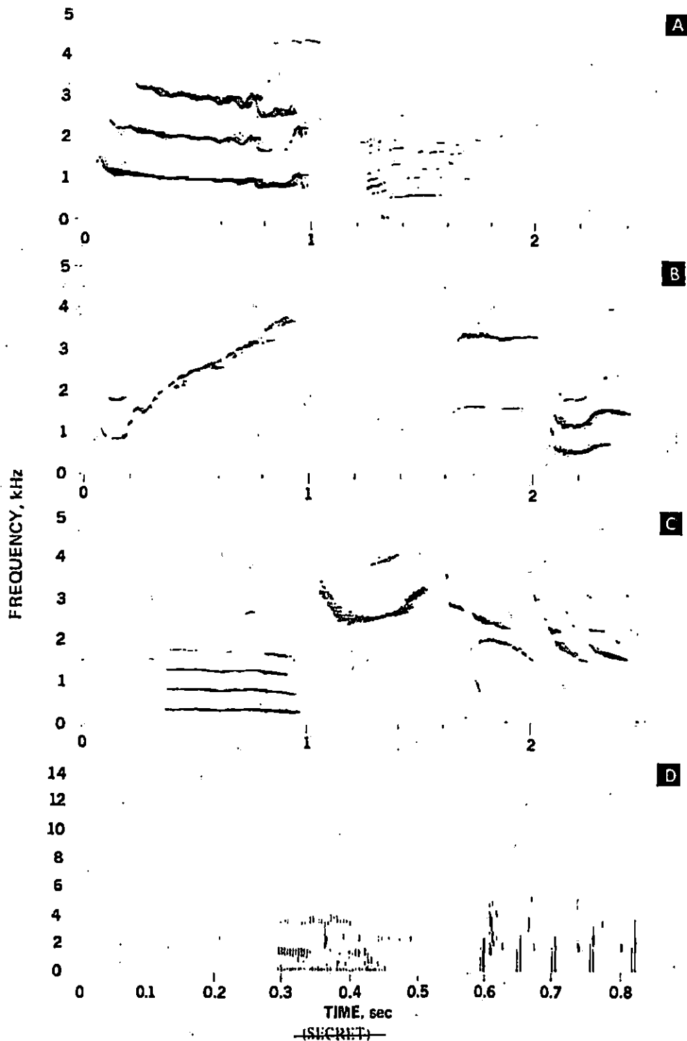
(S) Figure 2. Sonograms of sound with COMBO applications. A. beluga. B. killer whale. C. pilot whale. D. clicks of each, respectively. Effective analyzing filter bandwidth, 20 Hz (A,B,C.) 800 Hz (D).
