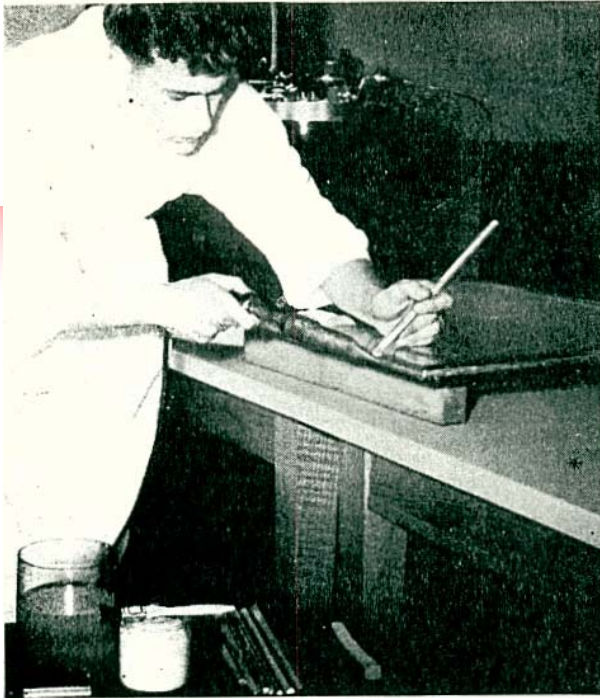
Figure 8.—Following the assembly of all enclosure elements, the lead strip is soldered to the glass plates in one of the most critical steps of the sealing operation. In the foreground are shown the soldering accessories used in bonding the lead strip to glass.
