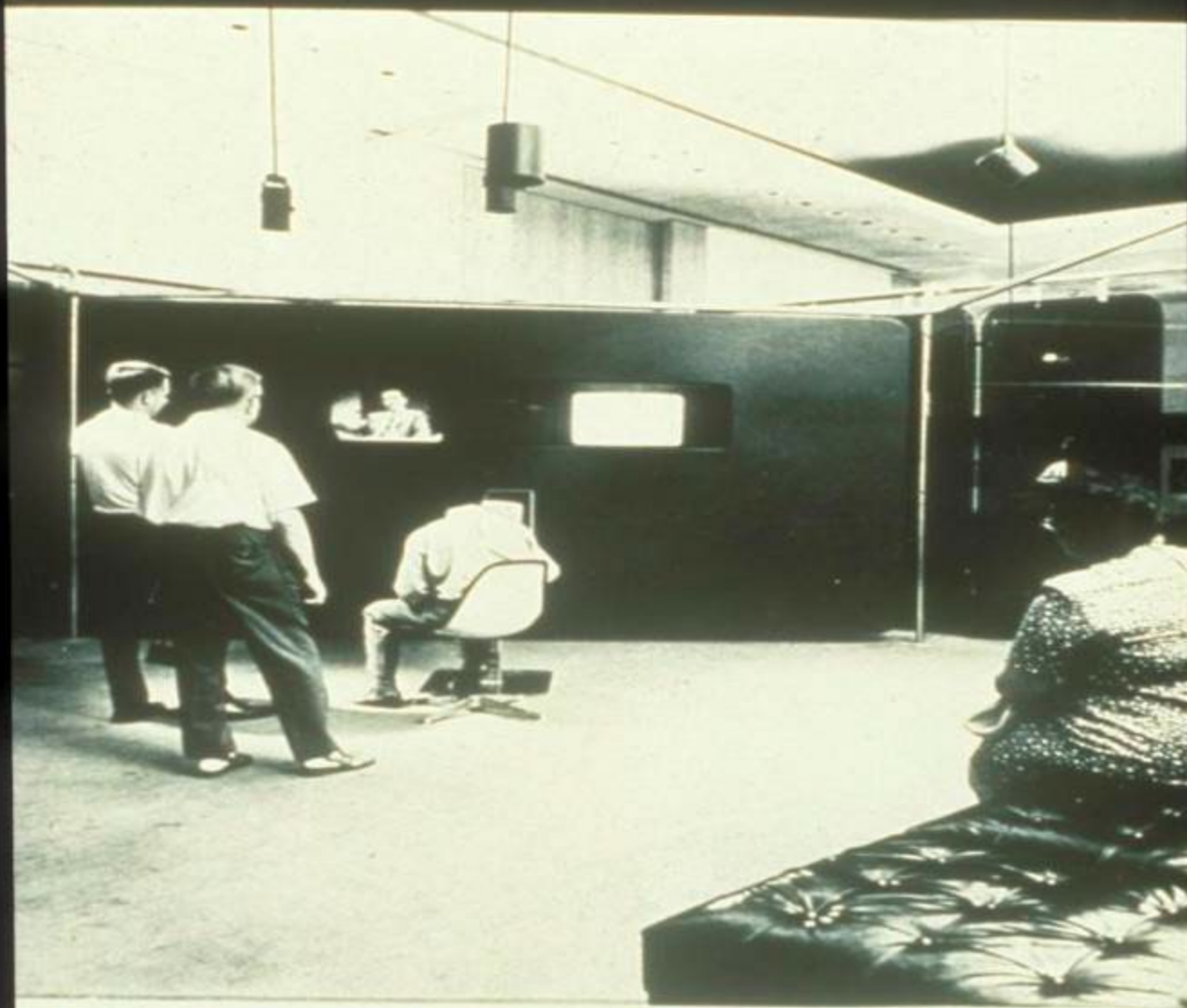
Fig. 1. Shows the exhibit in use a few days before the fire. A young visitor is shown operating the IBM-2260 keyboard/display console. The visitors are watching the display panel, or the front of the exhibit "wedge". The "wedge" houses the IBM 1051 terminal, a television display, projectors, and associated audio, signal and electrical equipment.
